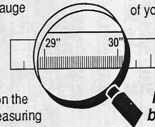
The electronic vacuum gauge, on the other hand, is measuring that last inch of pressure in 25,400's of an inch increments.
